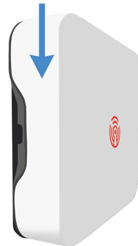
*Tip: apply pressure to the front of the device while pushing downward to help guide it straight into position.*
