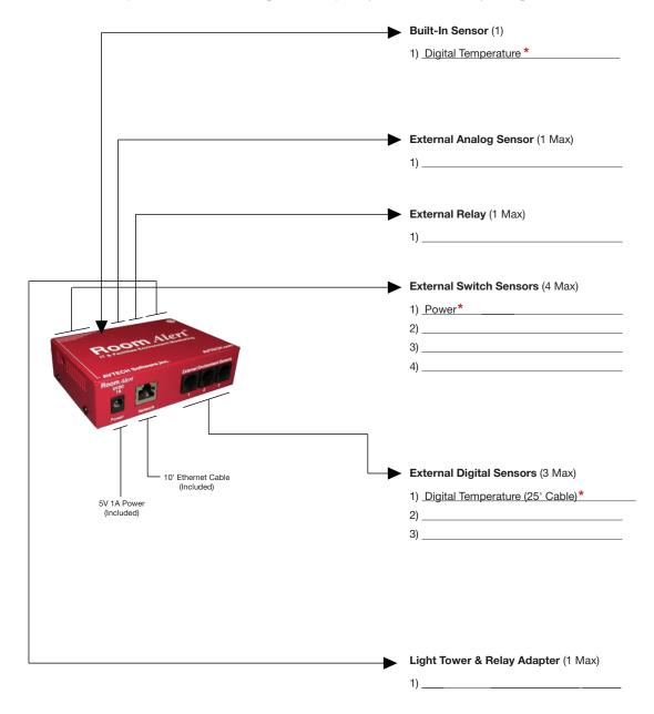
Note: The total sensor capacity of the Room Alert 12E is 11+ sensors.
