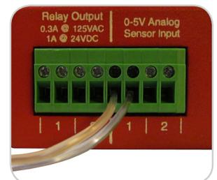
4. Insert the positive (+) wire into the LEFT (+) contact of the Analog Sensor Input port.
