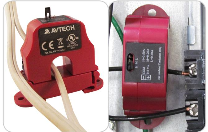
5. Lock the Current Loop closed by pressing the cover down firmly and listening for the click.
